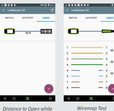
Distance to Open while connected to Switch
